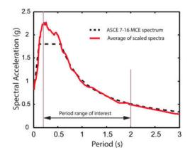
Figure 4. Scaling of the selected ground motions for the 6-story building
