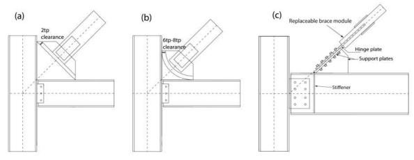
Figure 1. Brace to frame elements connection details: a) Typical gusset plate with linear hinge zone b) Typical gusset plate with elliptical hinge zone c) New proposed connection with replaceable brace module
