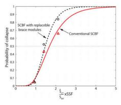
Figure 7. Collapse fragility curves
