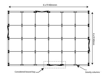
Figure 2. Plan configuration of 6-storey building
